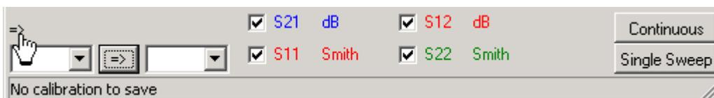
▶▶▶ **Note:** Without usage of an **S-parameter test set** the direction menu only determines, in which data spaces the measured data is stored. The function of the Tx port and Rx port remains unchanged. This means, **the VNWA2.x cannot automatically alter the signal flow direction.**
