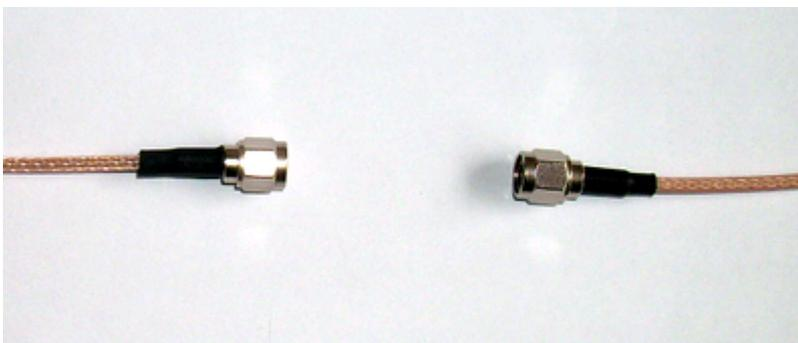
In case you run the "**Crosstalk Cal**", just leave the two cables separated from each other as shown above.
