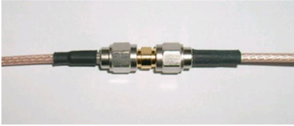
Note that the adapter introduces some phase shift because of its finite electrical length that has to be accounted for in the further reflection calibration.
