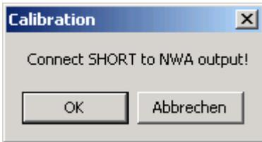
Now, connect the calibration standards, which you are asked for, and press ok when done. Output is synonymous for TX port and input for RX port. If you press "abort", no measurement will be performed. You can repeat any calibration measurement at any time. You can calibrate in any order you like. After a successful calibration sweep, the corresponding red lamp turns green indicating, that valid calibration data is available:
