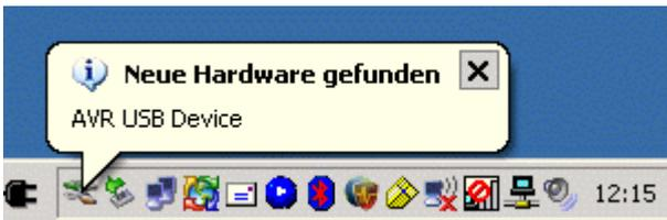
▶▶▶ **Hint:** In case Windows does not detect your USB\_VNWA interface, continue with the USB troubleshooting guide. In case Windows does not start driver installation automatically, proceed with manual driver installation via Windows device manager as is described in Example 4: Installing the LibUSB driver on Windows 7 (German screenshots).
