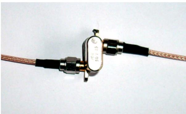
The only remaining problems are, that your reference plane still sits at the position where the end of the Thru adapter was, which would be well inside your test object now., and, in case of a two port calibration, your thru adapter for the thru calibration step should have been twice as long as it actually is. Both effects can be compensated in the port extension menu invoked by "Measure"->"Port Extensions":
